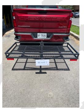
The Beast 2 is safe and easy to load and unload from the receiver and easy to lift up into a folded position against the back of your vehicle. With a single pin, the platform will pivot up and out of the way.
